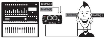
When connected to a stereo source, engage Stereo Mode. This will send the Left and Right input signals to their corresponding headphone output channels. While Stereo Mode is active, the pan control will adjust the stereo balance.
