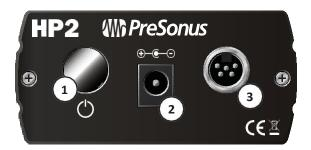
● Power Switch. Switches the HP2 on or off. ② DC Input Jack. Allows connection of the DC power supply. When a battery is installed in the unit, it is switched off as soon as the external power supply is connected. When the power supply is removed the unit will again run on battery power. ③ Input Connector. Allows connection of the 5-pin, mini XLR end of the supplied input cable. The opposite end of the input cable provides two female XLR jacks to connect to a source.
