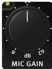
The gain control adjusts the preamplification. The control range ranges between +8 und +62 dB.
