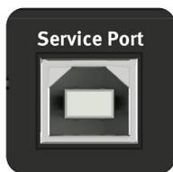
The service port (USB) on the optional AD converter of the P8 ensures that the digital interface can be easily maintained. It is used to transfer the operating software (firmware) and is not intended for audio connections.
