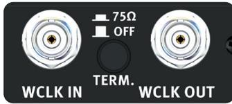
The word clock connection panel of the optional AD converter contains one clock input and output each as well as a switch for terminating the clock input.
