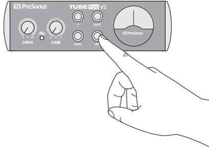
5. Speak into the microphone while watching the VU meter on the front panel and slowly turning the TubePre V2 Gain knob clockwise.
